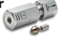
enters the small vessel volume and gauge through the capillary and is trapped momentarily thus "smoothing" out the pressure pulse. A stainless steel filter (20 micron) is included at the entrance of the capillary to prevent dirt or foreign objects from clogging the small bore of the capillary.
