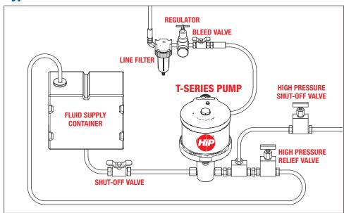
NOTE: T-Series Pump is the only item supplied by HiP with order of pump. All other components are available from HiP to be ordered separately.
