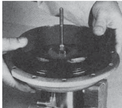
Figure 7-7 Pressing cylinder into lower housing.
