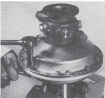
Figure 4-6 Removing housing screws and nuts.
