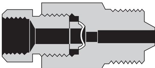
The male inlet design can be inserted directly into the tubing connections of valves and various fittings such as tees and crosses, or located in pressure vessels.
