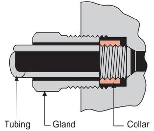
**Materials.** All of the components required for make-up of a Medium Pressure connection (glands, collars and plugs) are produced in Type 316 stainless steel.
